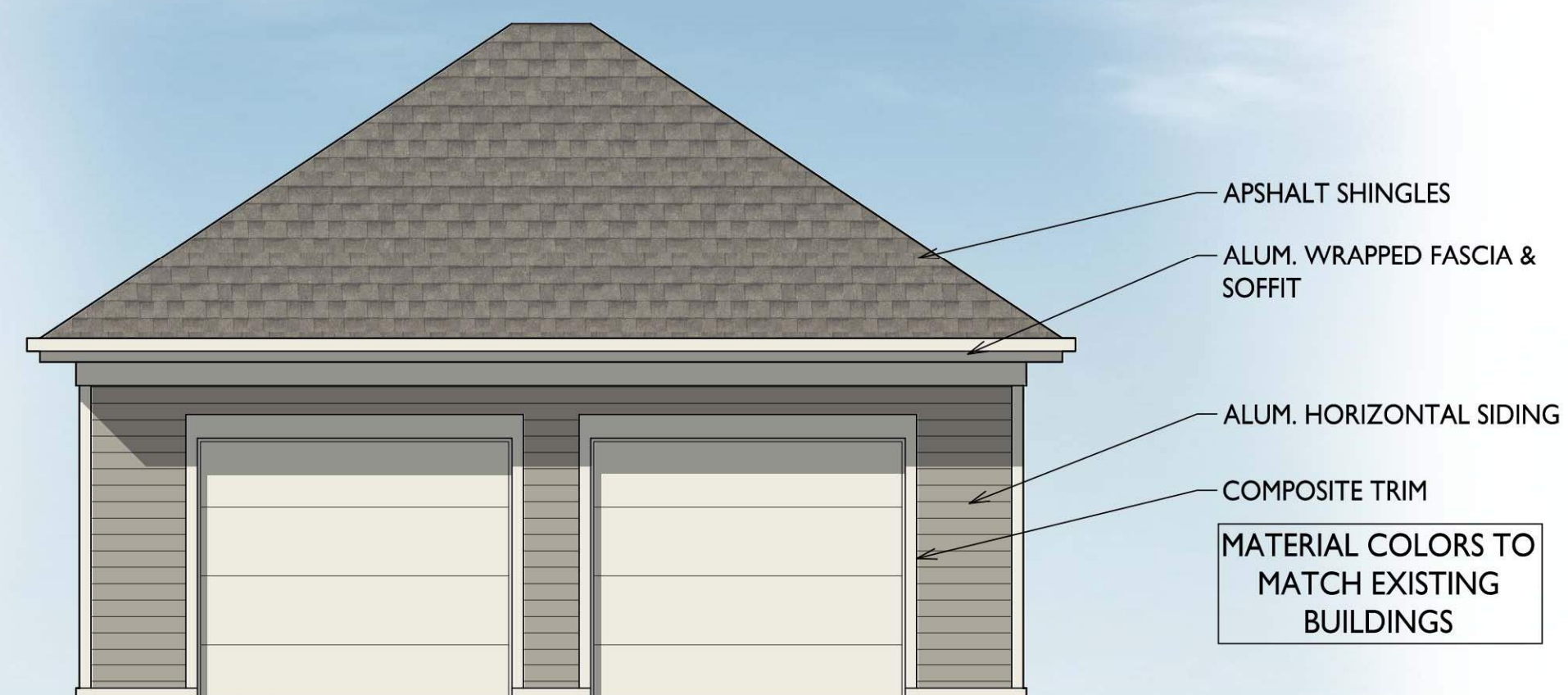
BUILDING B- STORAGE SHED - FRONT ELEVATION
